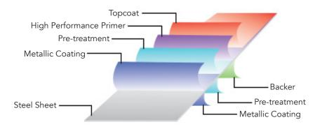
Metal Line Series<sup>™</sup> is manufactured from Canadian made Granite<sup>®</sup> Deep Mat (GDM). Coated 28 gauge, galvanized, recycled steel that is strong, light and durable. This Canadian made precoated steel is superior to other steel made off-shore.
